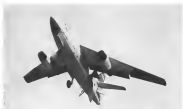
NAVY VERSION, A3D, similar to its landing on USS Forrestal. Wing sweepback of 16 deg. is same for both A3D B-66 but B-66 has extended center section leading edge.
